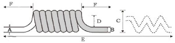
High Elasticity is a way that pull A to B from Coil hole to increase the elasticity. But it will affect length of using and could not have F tails.
